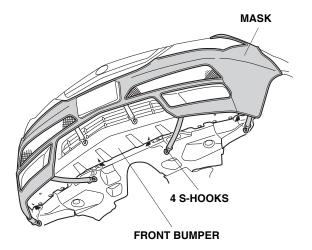
9. Attach the two S-hooks to the inside edge of the lower grille opening.
